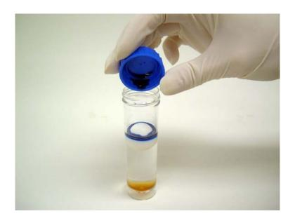
Once the methylene blue has been added to the tester, a blue band will appear (4 to 8mm) around the ball and down into the sample. Screw the cap firmly back onto the tester the tester and rotate the tester five times to ensure oxygenation of the sample and that the methylene blue has mixed into the sample (see also protocol DBHSOPO5 for more details of this procedure).
