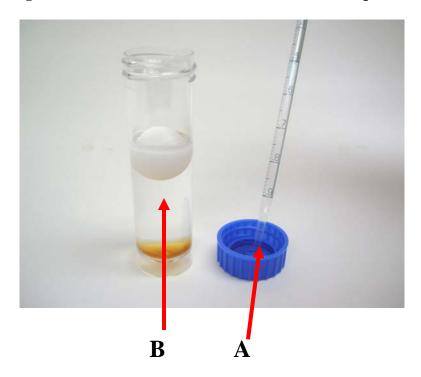
Plate Two, Once the 0.5mL of water has added then the cap is left for 30 seconds to dissolve the methylene blue and the contents of the cap are tipped into the tester.
